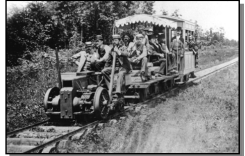
A locomotive and two passenger cars of Thomas Edison's experimental electric railway at Menlo Park. (from the U.S. Dept. of the Interior, National Park Service, Edison National Historic Site)
